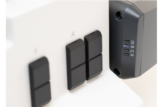
The lights at the Colibri 3 LED illumination indicate which channel you're using.
